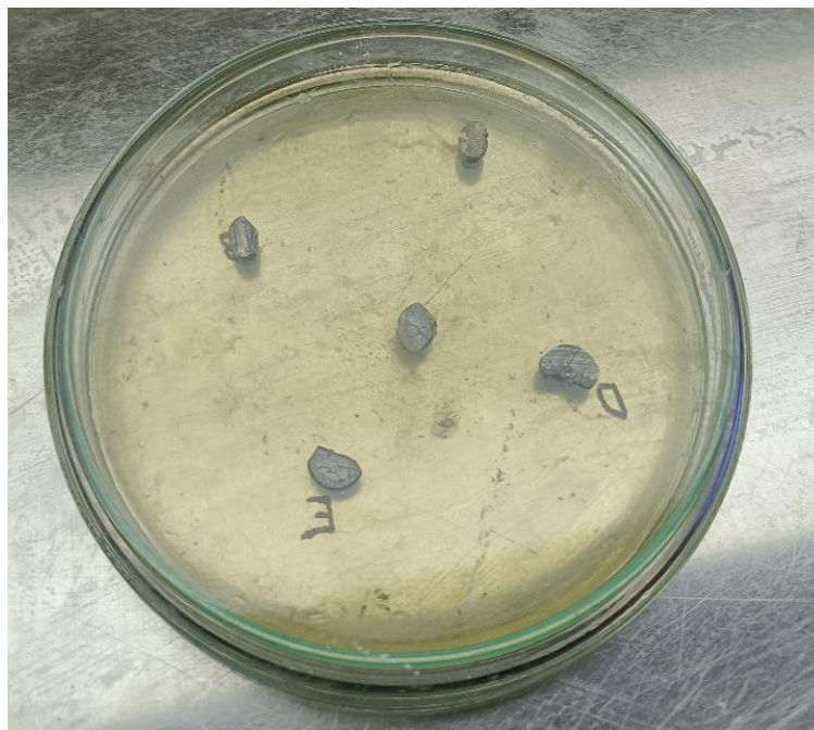
Figure 6.8: Agar Plate with \text{Ho}_4\text{PtAl} (A), \text{Er}_4\text{PtAl} (B), \text{Ho}_2\text{RhSi}_3 (C), \text{Nd}_2\text{RhSi}_3 (D), \text{Er}_2\text{RhSi}_3 (E) sample disks
