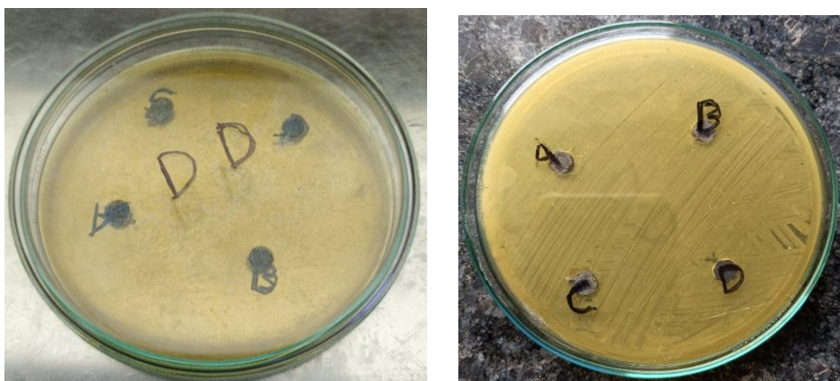
Figure 6.13: Left image shows agar plate with wells filled with Dy_4RhAl (A), Ho_4PtAl (B), Er_4PtAl (C) and Ho_2RhSi_3 (D) on day 0 and right image shows the growth after 28 hours of Incubation at 37^\circ C for P. Acne .
