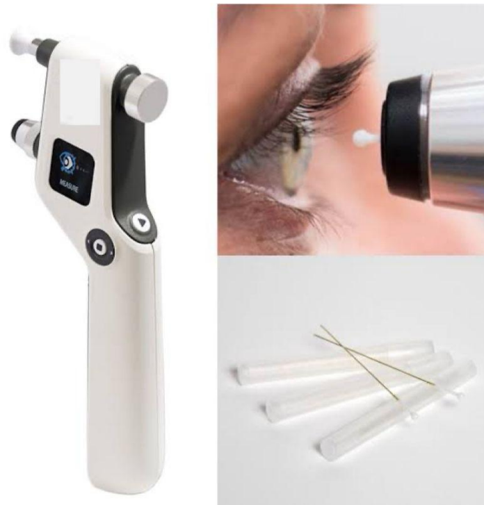
Figure 15: Usage of Rebound tonometry (iCare website (32))
