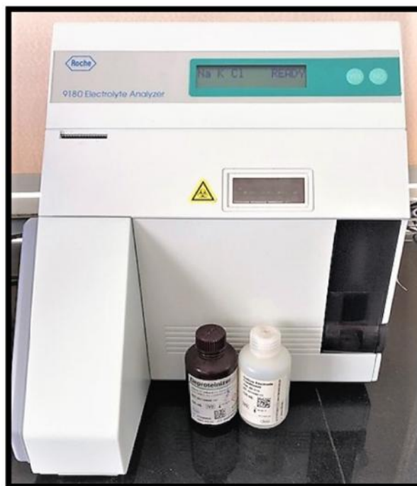
Photograph 2: Roche 9180 Electrolyte Analyzer by ARK diagnostics Pvt. Limited for the estimation of serum electrolytes.
