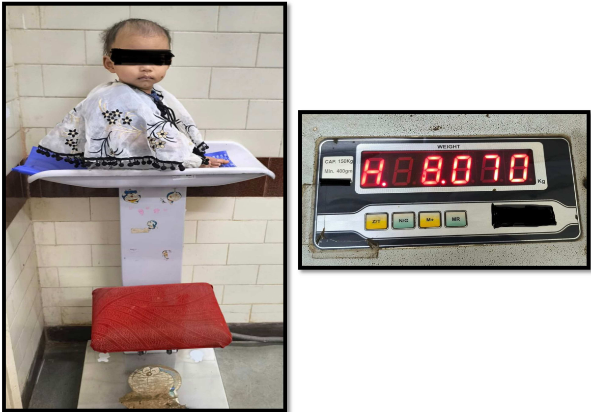
Photo 3: Multipurpose digital weighing scale ranging from 50g to 120kgs with 5g division was used (meditive brand)
