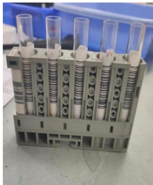
4. After serum separation the samples are arranged in sample rack for placing the rack in the analyser before estimation
