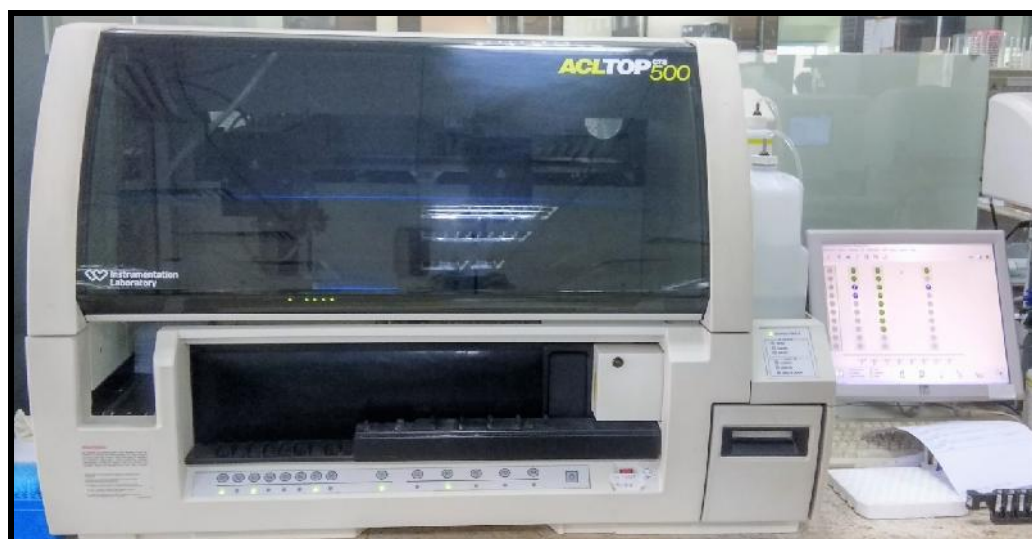
Photograph 6: Instrumentation Laboratory's ACL Top 300/500 used for estimation of D Dimer levels
