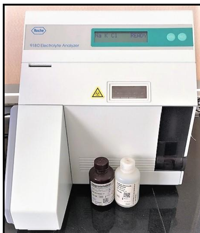
Photograph 5 : 9180 Electrolyte Analyzer used for estimation of serum electrolytes
