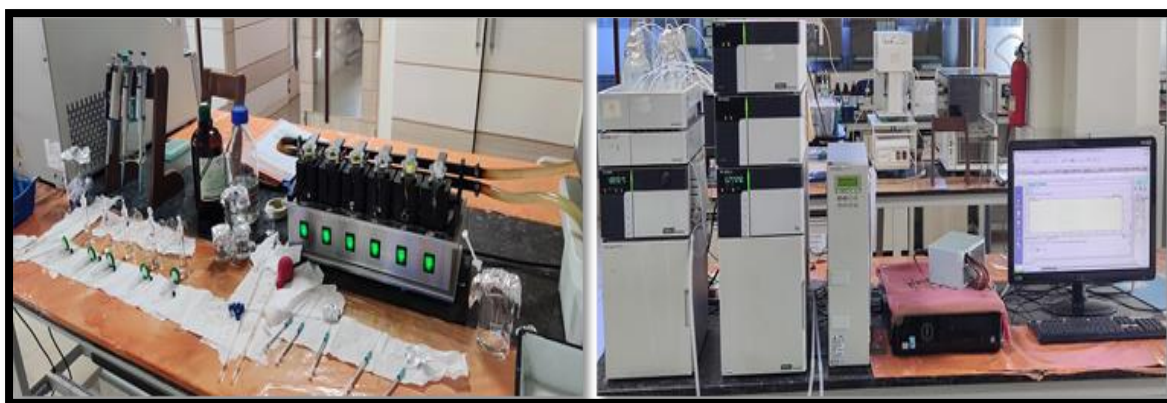
Figure 4. Permeation study setup: Franz diffusion cell apparatus (PremeGear, USA) and RP-HPLC instrument (Shimadzu, Japan).
