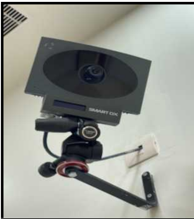
FIGURE 5: SMART-DX 6000 CAMERA: HIGH PRECISION OPTOELECTRONIC SYSTEMS FOR MOTION ANALYSIS
