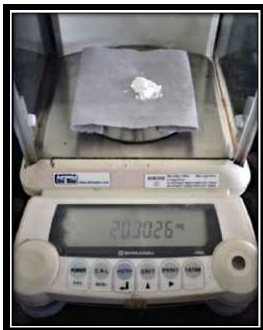
Fig 10: 2 g of Chitosan powder weighed by placing it on top of filter paper
