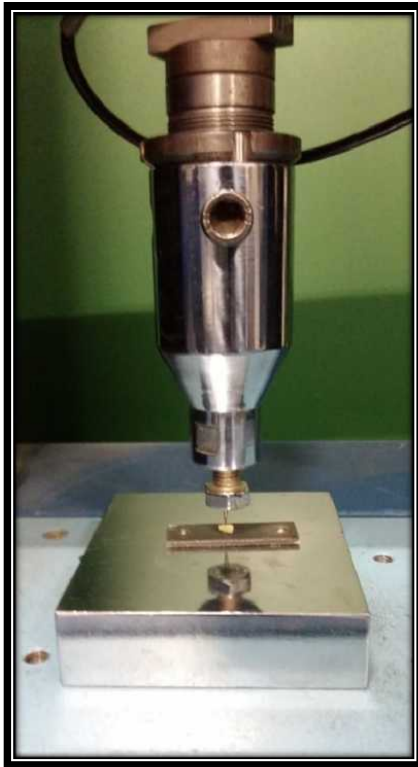
Fig 22: Pushout bond strength testing done using a Universal testing machine at a cross head speed of 1mm/min.
