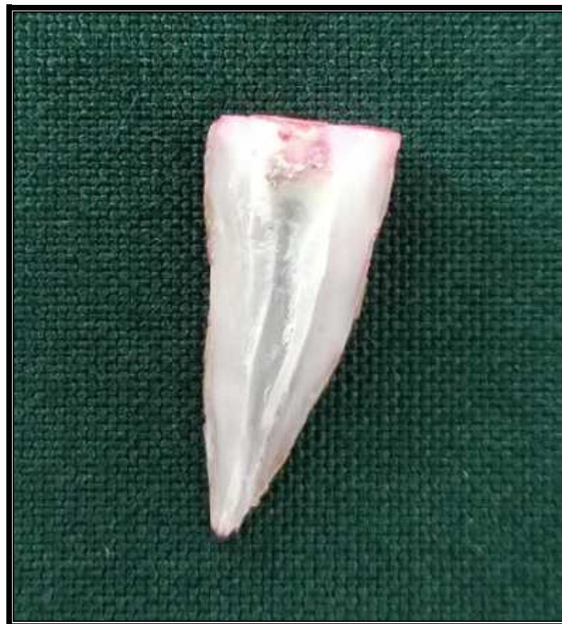
Fig 8: Teeth longitudinally sectioned and dye penetration observed
