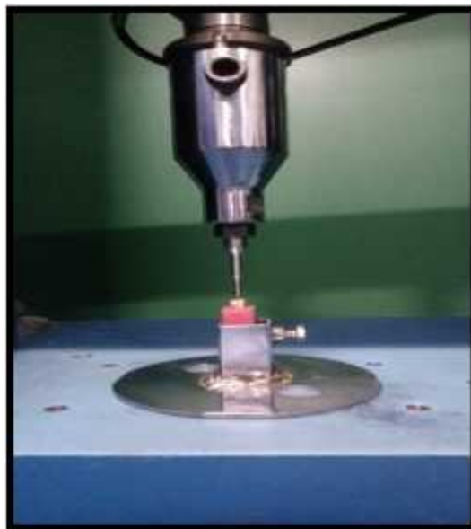
FIGURE 26: Fracture resistance testing using universal testing machine
