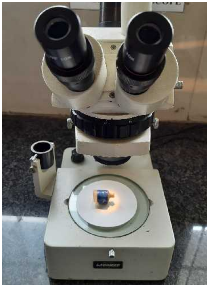
FIGURE 10: SAMPLE EVALUATED UNDER STEREO MICROSCOPE TO MEASURE ARI
