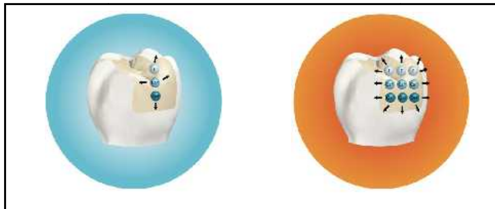
Figure No.2: Schematic representation of low (left) and high (right) levels of calcium, fluoride and hydroxyl ion release, depending on the pH in the oral cavity
