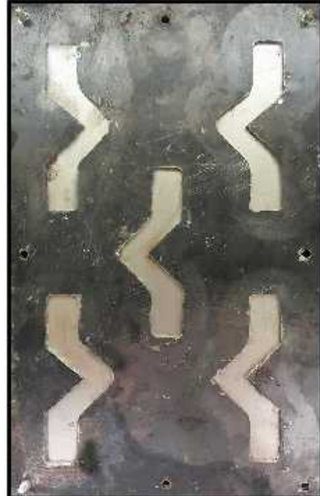
Fig 15. Mould for preparation of Tear test samples. (ASTM D264)
