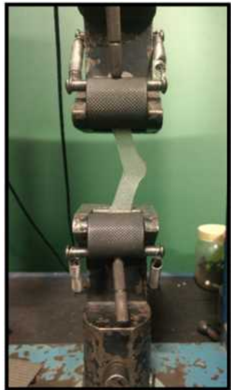
Fig. 31, 32 Sample subjected to universal testing machine for tear strength test
