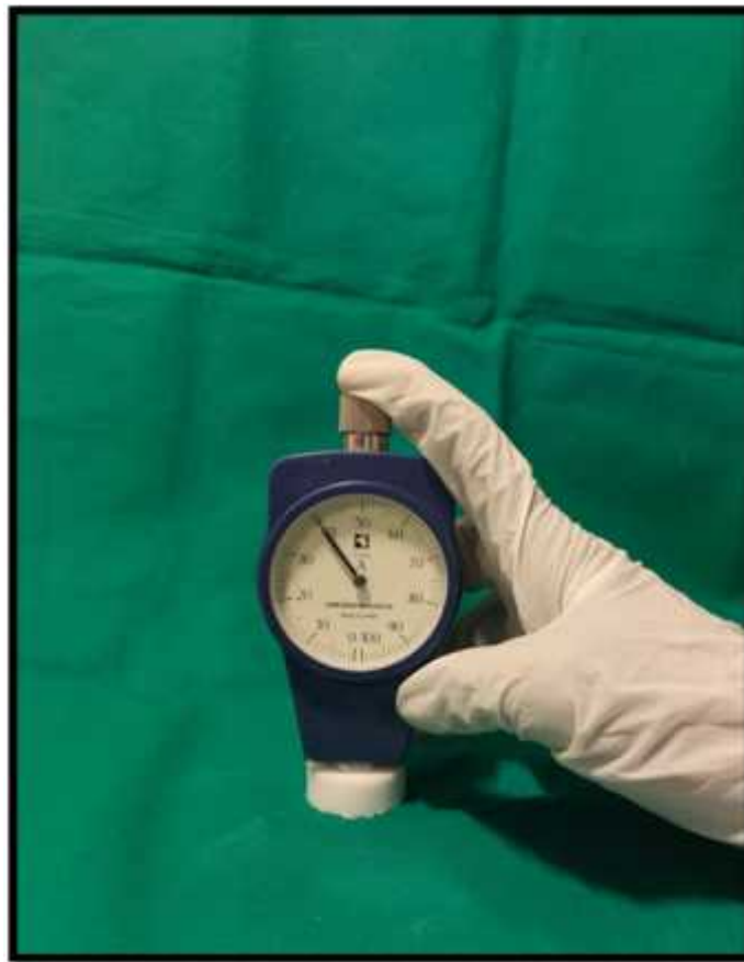
Fig. 33, 34 Sample subjected to a durometer testing machine for hardness test.
