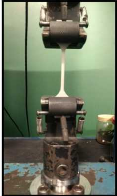
Fig. 29, 30 Sample subjected to universal testing machine for tensile strength test
