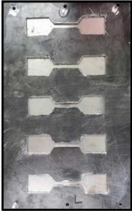
Fig 14. Mould for preparation of Tensile test samples. (ASTM D412)
