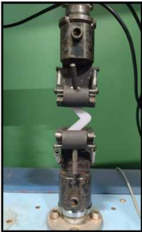
Fig. 31, 32 Sample subjected to universal testing machine for tear strength test
