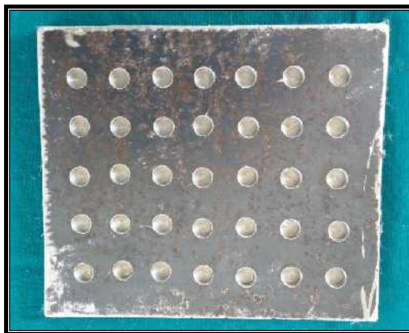
Figure 4: Metal mould for fabrication of specimens
