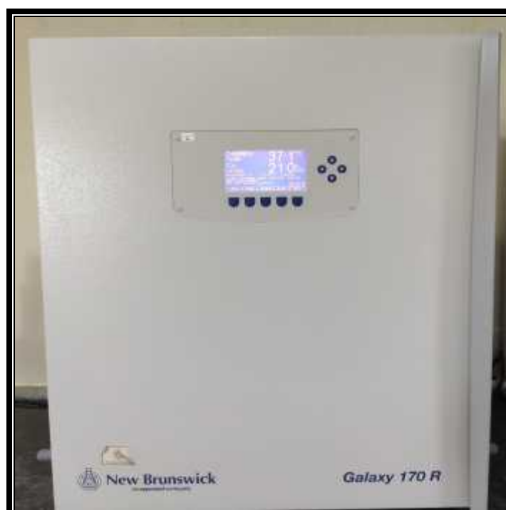
FIGURE 24: CO 2 Chamber for incubation of cell lines after the addition of MTT
