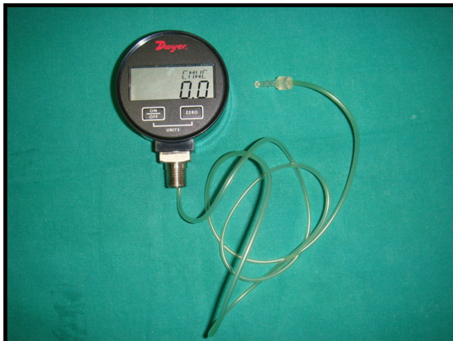
Photograph 6. Cuff pressure manometer
