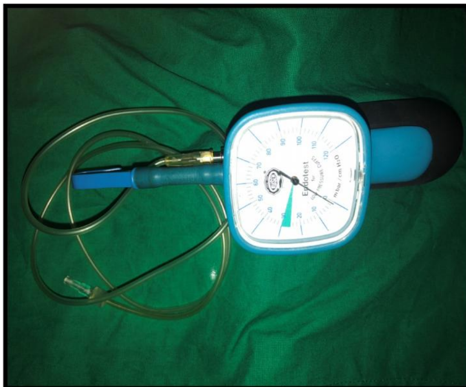
Photograph 8: Cuff pressure manometer
