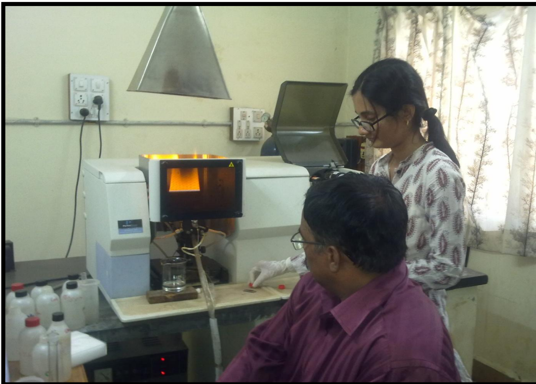
Photograph 2: Investigator performing analysis of lithium on Flame atomic absorption spectrophotometer (Perkin Elmer Analyst 300).
