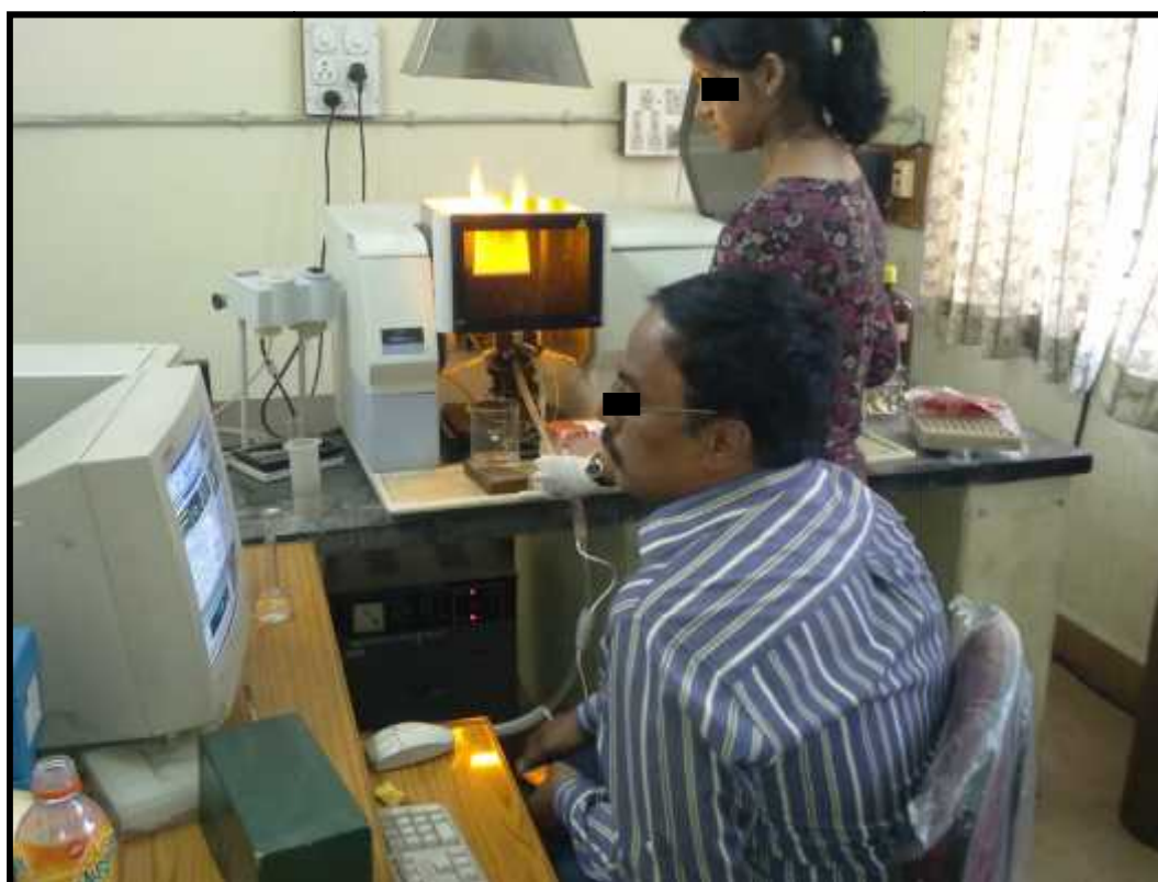
Photograph 4: Investigator performing analysis of serum zinc on Flame atomic absorption spectrophotometer (Perkin Elmer Analyst 300).
