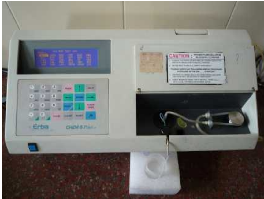
Photograph 1. Semi-Auto Clinical Chemistry Analyser machine (ERBA Chem-5 Plus) used for LFT
