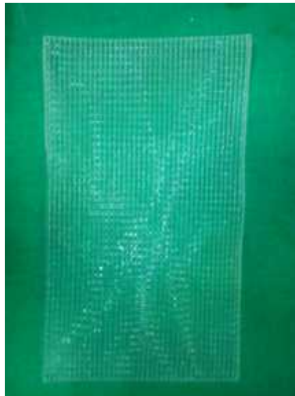
Photograph 10. The heavy weight composite polypropylene mesh. Microporous knitted polypropylene mesh with pore size of 75 micrometer and prolene content of 95-100ng/m 2
