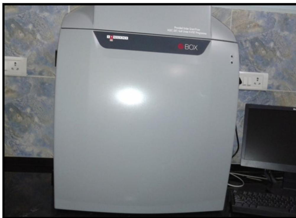
PHOTO 8 : Syngene Agarose Gel Documenttion system used to read and record the results of agarose electrophoresis.
