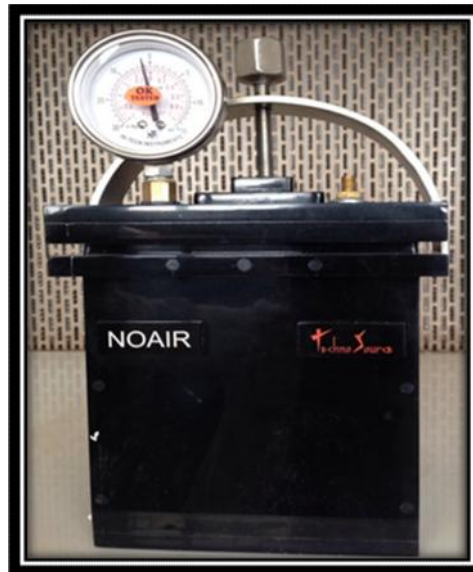
Photograph 7: McIntosh Filde's anaerobic jar
