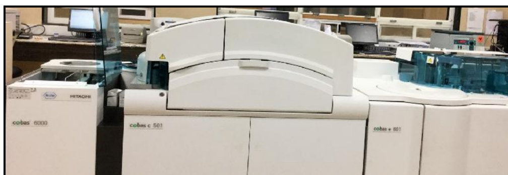
Photograph 4: Cobas analysers for quantitative measurement of serum procalcitonin and serum c-reactive protein
